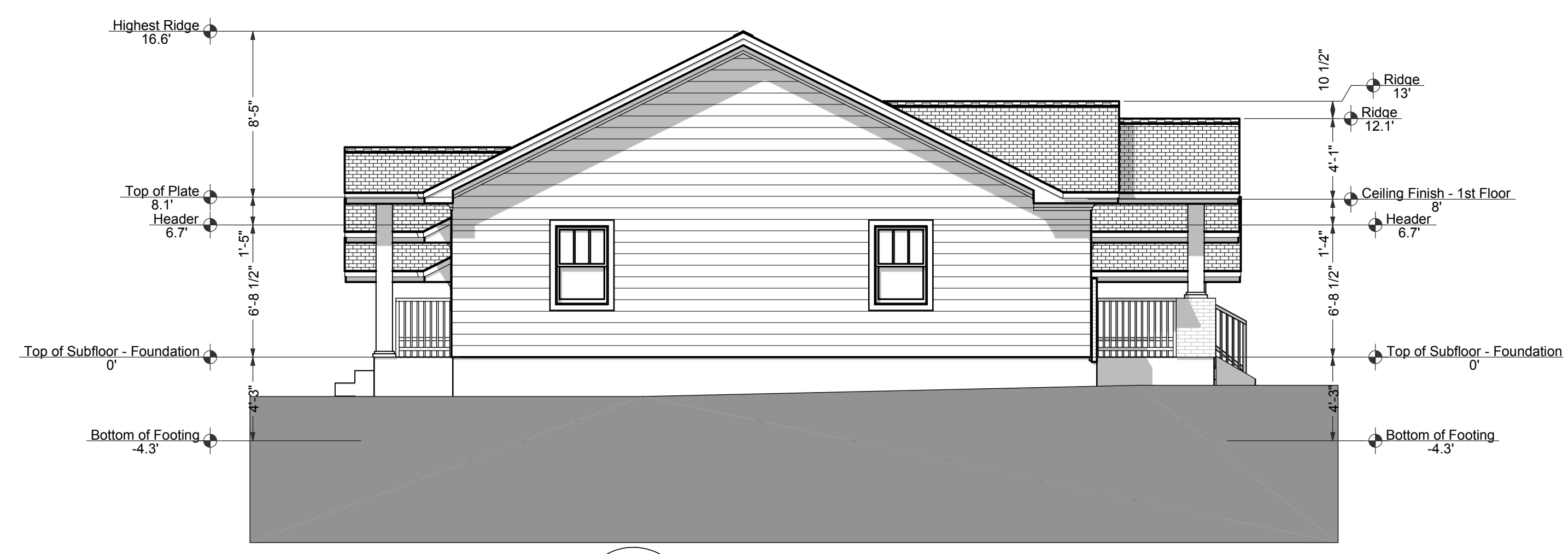
BE3 Building Elevation 3 A20 3/16 in = 1 ft
