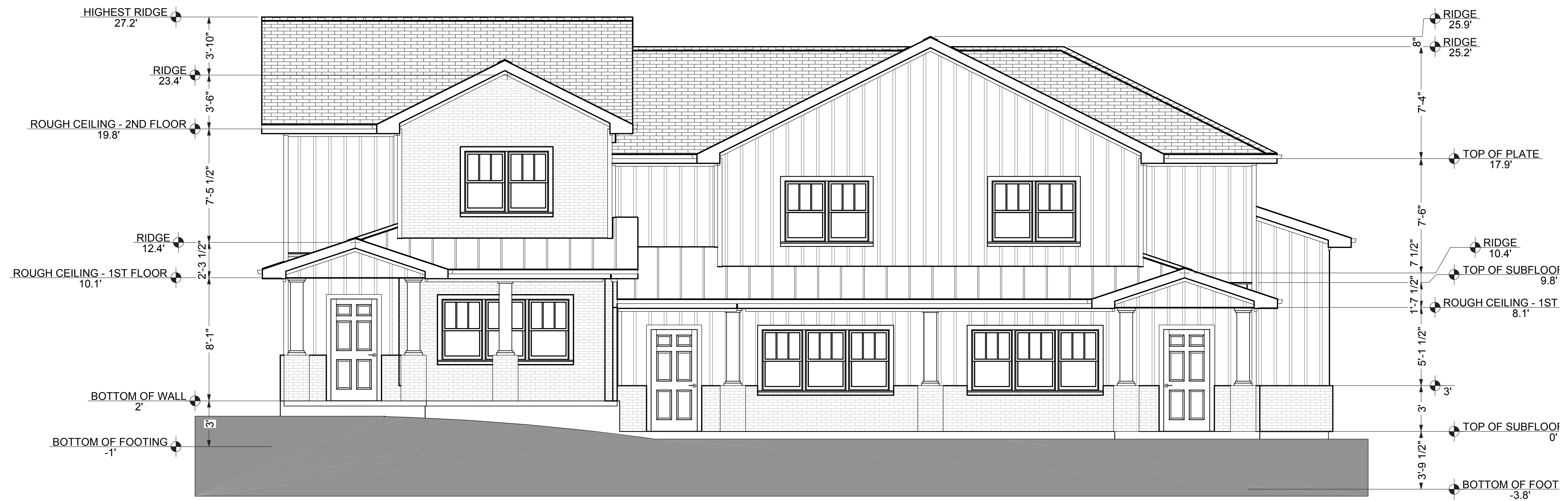
BE1 Building Elevation 1 A5 1/4 in = 1 ft
