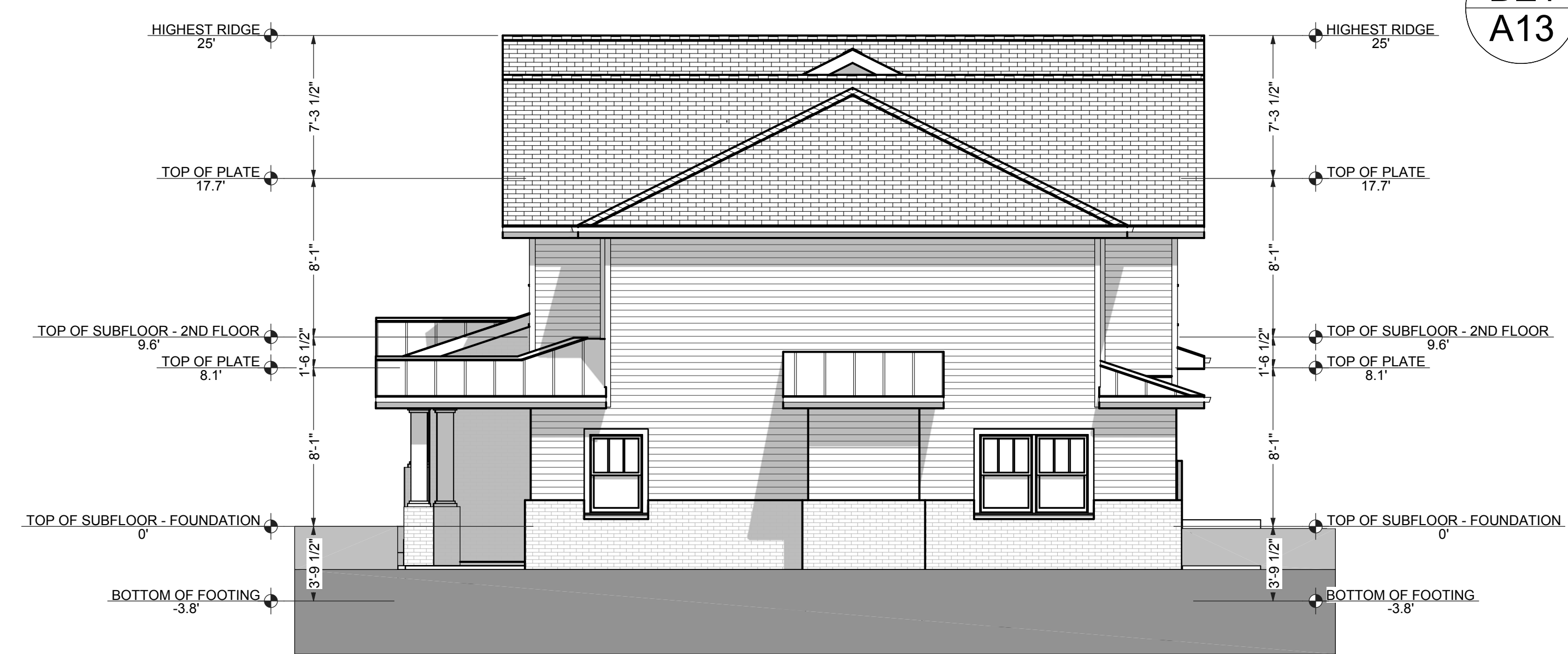
BE2 Building Elevation 2 A13 3/16 in = 1 ft
