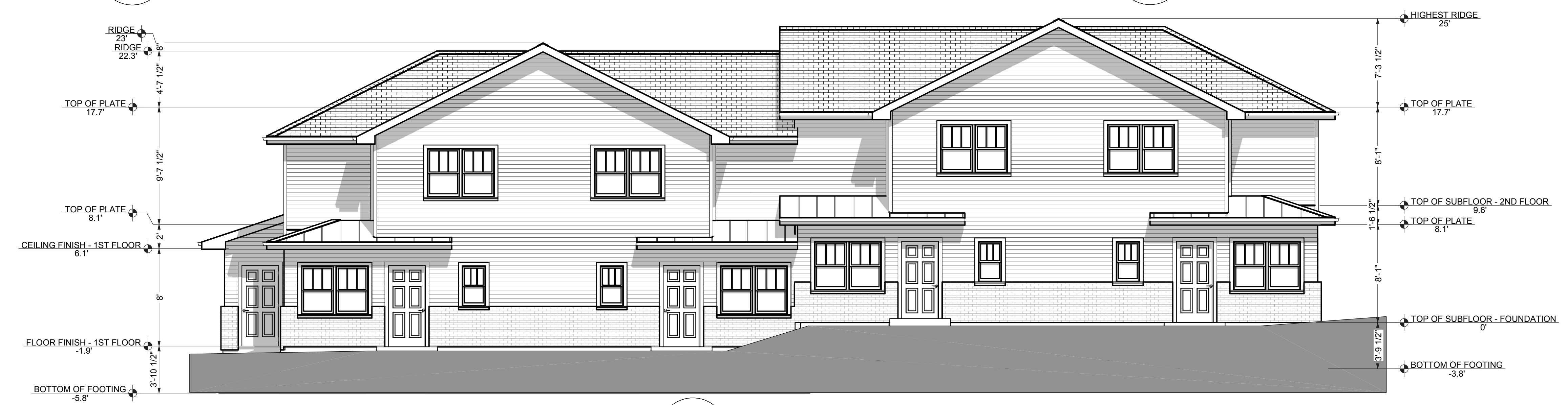
BE4 Building Elevation 4 A13 3/16 in = 1 ft
